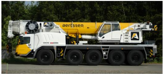
Specifications: CRANE 100 TON + extra ballast if needed! width 2.99M Length 12M with crane arm 13,3 M width crane stabled with stamps in Position 7,5M length arm 11,7 - 60M
