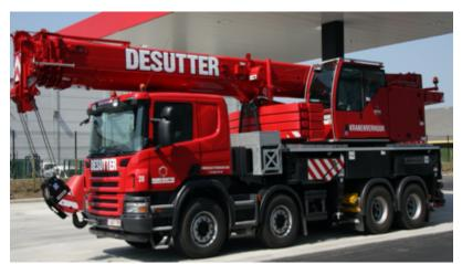
Specifications: CRANE 60 TON + extra ballast if needed! width 2.55M Length 9 M and with crane arm 11,5M width crane stabled with stamps in Position 7M length arm 9,6 - 43M
